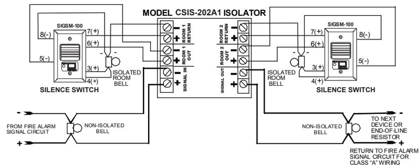
Figure 3: CSIS-202A1 Isolator wiring with SIGSM-100
