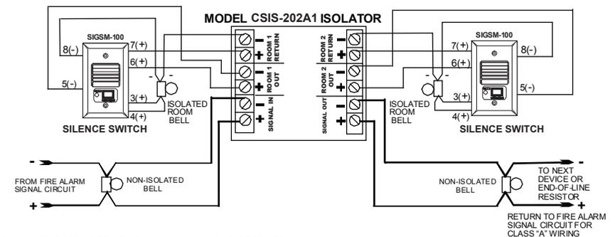
Figure 3: CSIS-202A1 Isolator wiring with SIGSM-100
