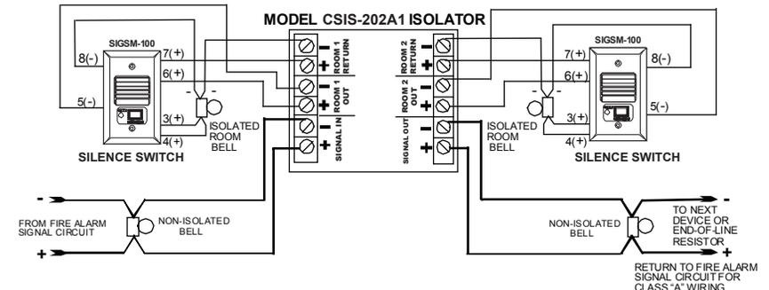
Figure 3: CSIS-202A1 Isolator wiring with SIGSM-100
