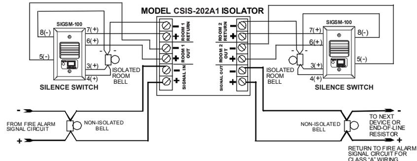
Figure 3: CSIS-202A1 Isolator wiring with SIGSM-100
